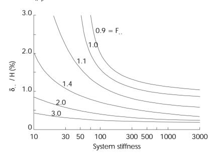
The maximum settlement  $(\delta_{vm})$  behind a retaining wall in soft clay is equal in magnitude to its maximum horizontal movement  $(\delta_{hm})$  and is given by:
