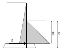
To simplify the analysis, the earth pressures acting below the pivot are replaced by a single resultant force (R). The depth of the pivot below excavation level  $(d_o)$  is given by:
