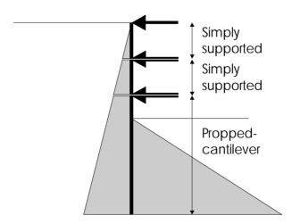
The simply-supported sections of the wall are inherently stable, but the propped cantilever section needs sufficient embedment in the ground to prevent the wall toe from kicking into the excavation.
