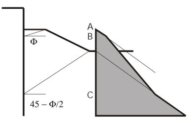
The increase in vertical total stress ( $\Delta \sigma_{v}$ ) due to the presence of a berm depends on whether it is *wide* or *narrow*.
