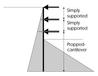
ReWaRD determines the structural forces in propped-cantilever section using one of the methods described above for cantilever and single-propped walls.
