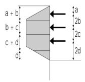
The load carried by the top prop is equal to the area of the first segment, of thickness a + b.
