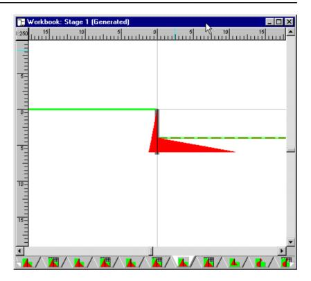
Note that the earth pressures on the excavated side of the wall *do* begin at formation level – this is because CIRIA 104 does not require a minimum unplanned excavation to be considered.
