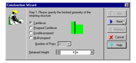
If not already selected, click on the **Cantilever** option. The number of props changes to 0 and the picture shows a cantilever wall.
