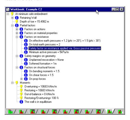
The minimum safe embedment for this wall is 15.5m, based on a
