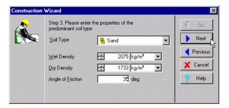
Select Sand from the **Soil Type** box; leave the wet density at its default value; and enter a dry density of 1733 kg/m³ (which is equivalent to 17 kN/m³) and an angle of friction of 35°.
