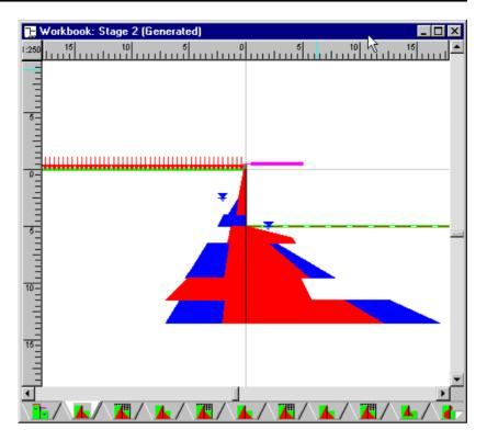
Note how the earth and water pressures change with the various layers in the ground. Note also how the passive earth pressures drop to zero at formation level on the excavated side, owing to CIRIA 104's required for a 1m softened zone.
