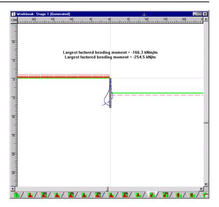
Bending moments are shown by a dark blue solid line and shear forces by a light blue dashed line. Maximum values of each are noted on the diagram (these are design values – i.e. they already include appropriate safety factors, which in the case of BS 8002 are 1.0). The dashed red line on the right hand side of the picture indicates the unplanned excavation that ReWaRD has applied in accordance with BS 8002.
