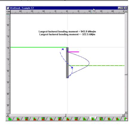
The maximum bending moment in this case is 944 kNm/m and the maximum shear force is 323 kN/m. These are design values – i.e. they already include the appropriate safety factors (which in the case of CIRIA 104 are 1.5).
