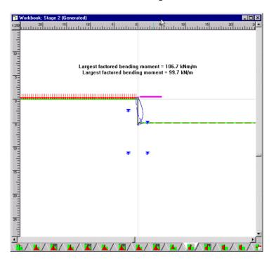
ReWaRD also provides the results of the structural forces calculations in a table or spreadsheet. To view the results in this format, choose the **Table** command from the Workbook's **View** menu.
