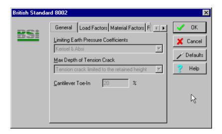
Click on each of the tabs in turn to see what rules the program follows when it performs its calculations. In particular, note the partial factors that are applied to the soil's drained parameters.
