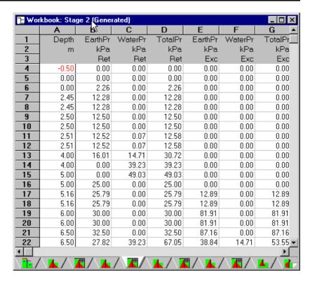
By default, ReWaRD displays the design pressures on the wall (see the *ReWaRD Reference Manual* for further information.) You can change what ReWaRD displays in the table by choosing one of the commands on the bottom half of the **View Earth Pressures** fly-out menu:
